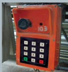
Local telephone network inside TBM
