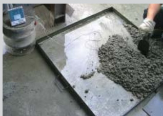
The temperature of concrete for making precast segments is kept below 32°C
