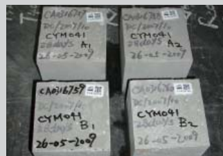
To ensure the concrete strength of the precast segments is up to standard, the concrete is tested in a laboratory
