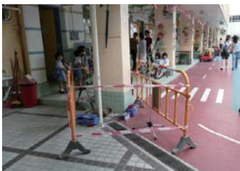
Vibration monitoring is carried out during blasting operation
