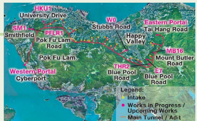
Layout plan for Hong Kong West Drainage Tunnel
