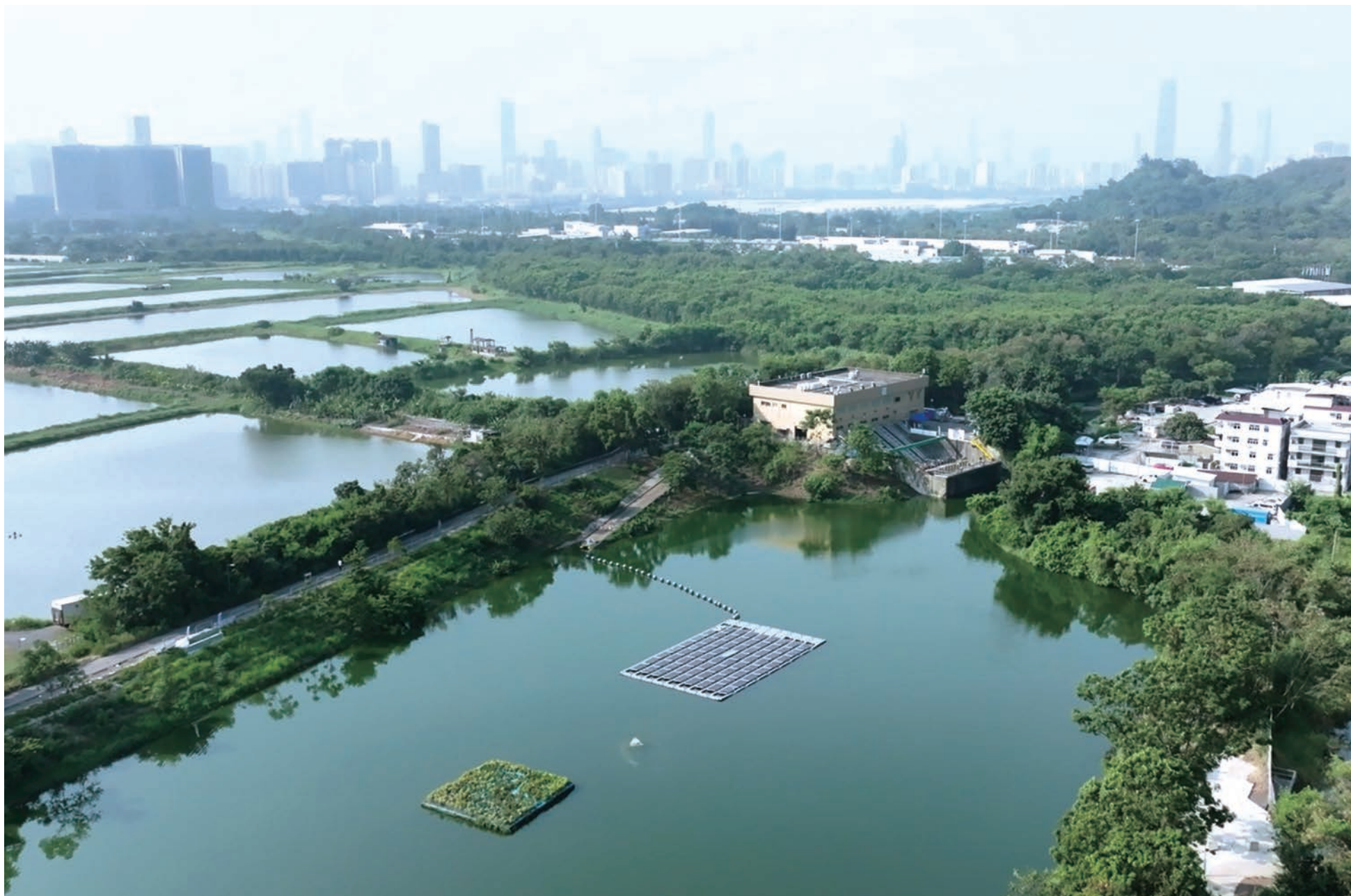
For sustainable development, floating photovoltaic system and ecological floating island are installed in San Tin Polder in 2022. 為可持續發展，新田蓄洪池在2022年安裝浮式太陽能發電系統和生態浮島。
