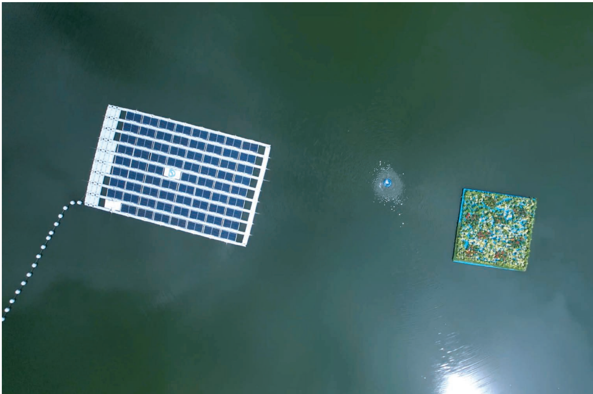
Aerial view of San Tin Polder with a floating photovoltaic (FPV) system and an ecological floating island 配備浮式太陽能發電系統及生態浮島的新田蓄洪池鳥瞰圖
