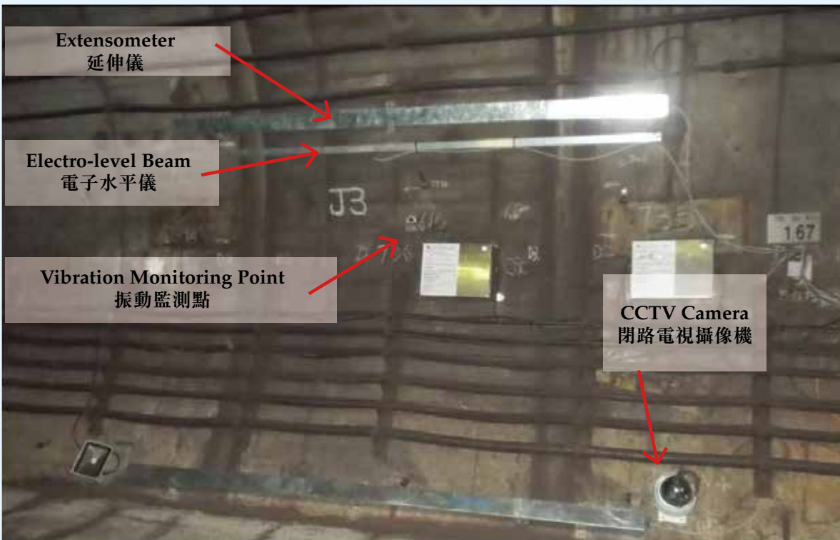
Devices installed in MTR tunnels for monitoring the blasting underneath 於港鐵隧道內安裝儀器以監測隧道下的爆破工程
