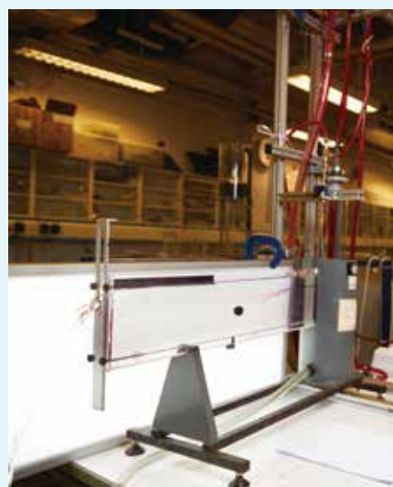
Hydraulic model for optimisation of disinfection facilities in SCISTW 用以優化昂船洲污水處理廠消毒設施的水力模型
