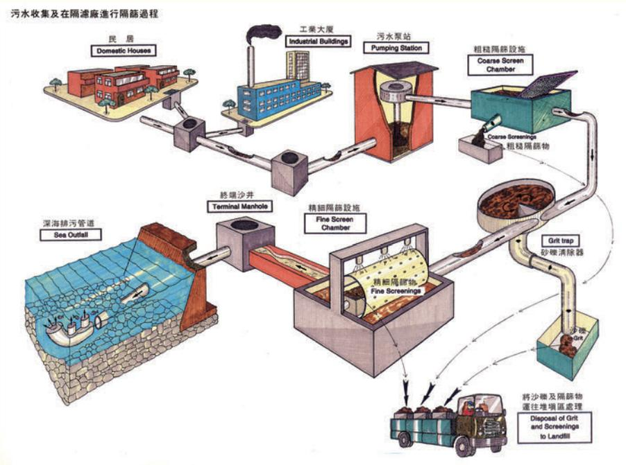
Typical operation flow within a preliminary treatment plant
