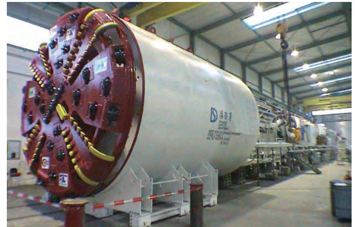
The tunnel boring machine used in constructing the Kai Tak transfer tunnel
