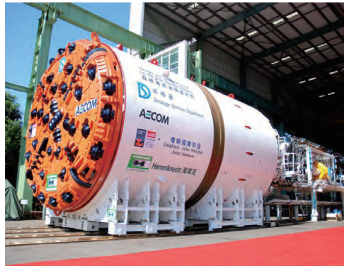
The “mixshield slurry type” tunnel boring machine
