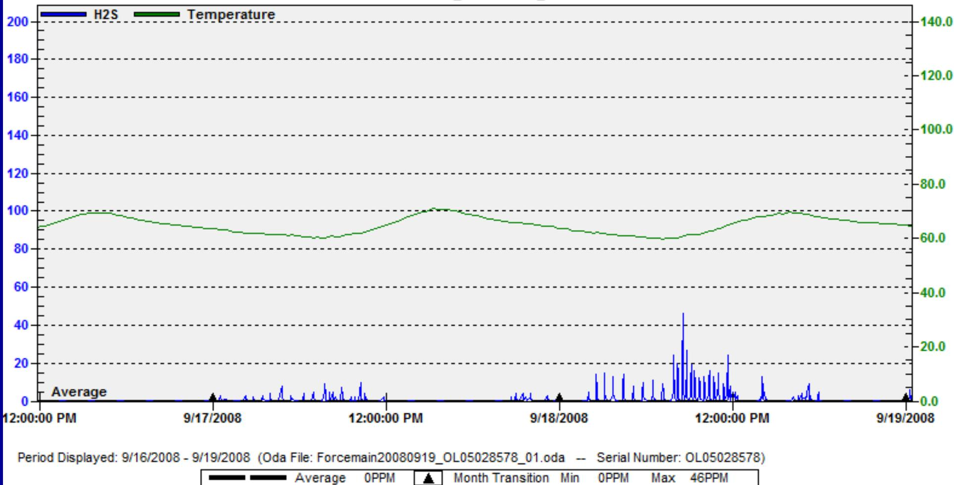
H<sub>2</sub>S levels in forcemain discharge after O<sub>3</sub>/O<sub>2</sub> injection into wet well
