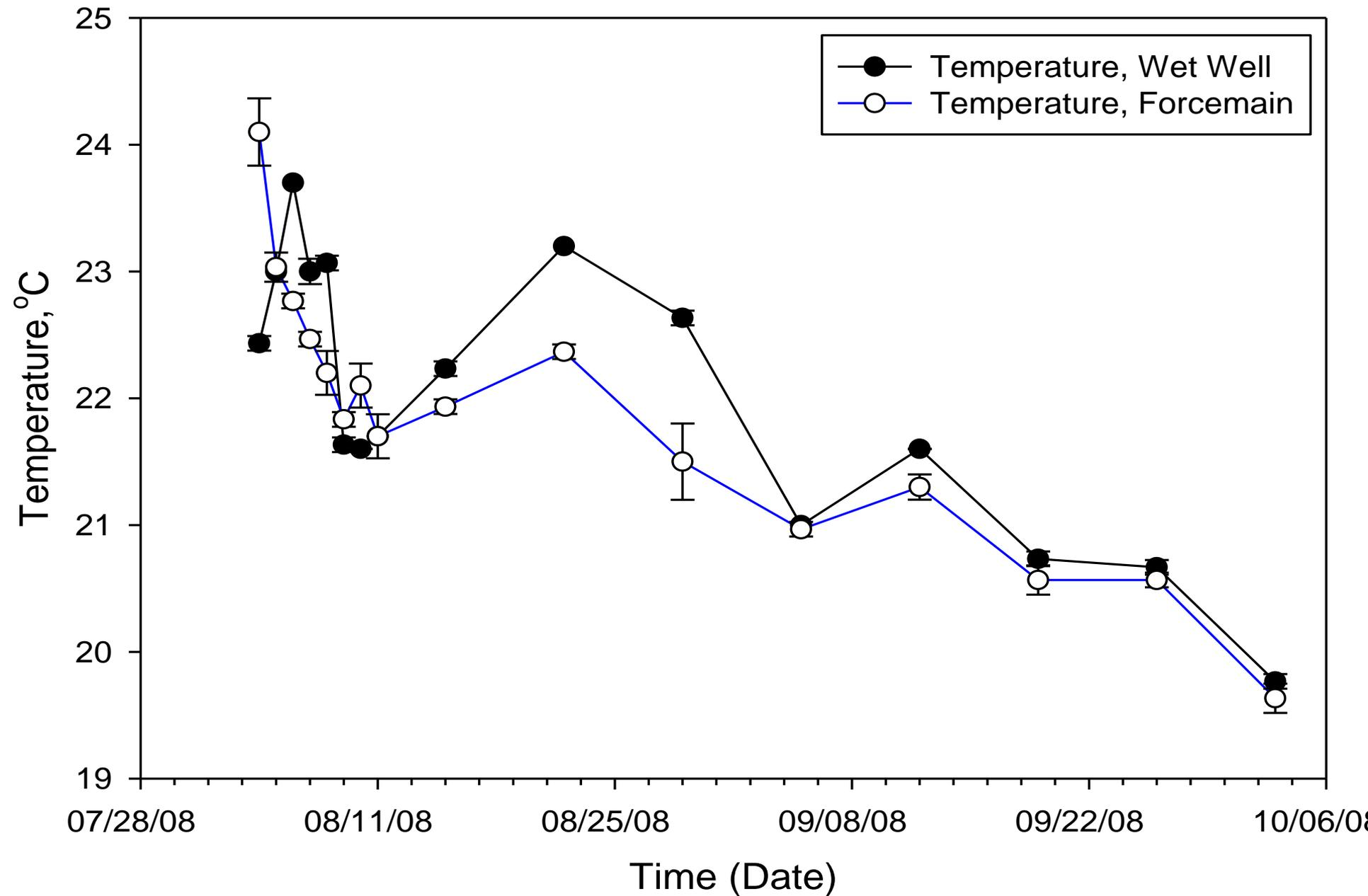
Fig 1. Wet well and forcemain temperatures
