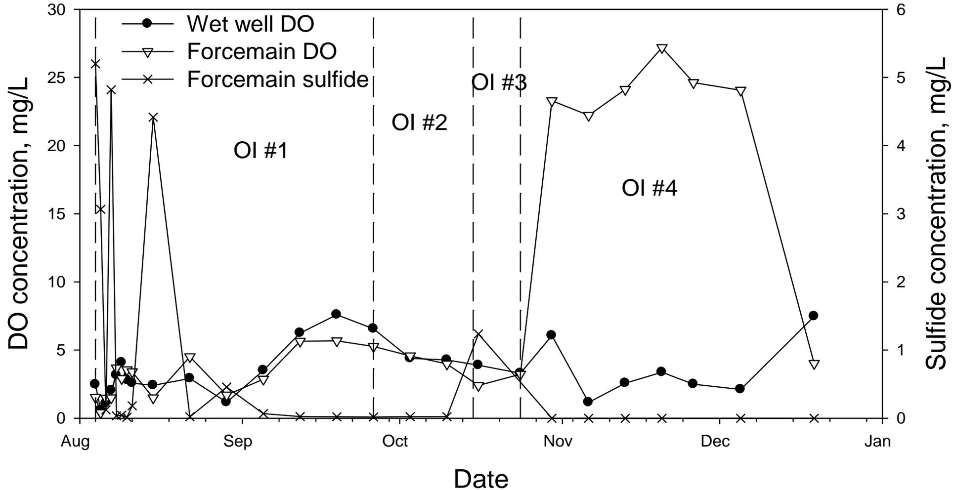
DO and sulfide concentrations in forcemain discharge
