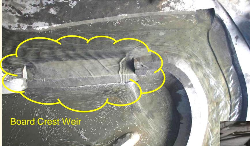
Shapes of weir and flow diversion wall optimised to achieve even and steady flow through the overflow weir
