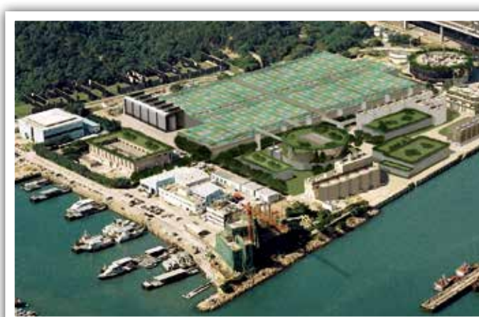
Works of HATS Stage 2A – covered sedimentation tanks of Stonecutters Island Sewage Treatment Works. (computer simulated photo)
