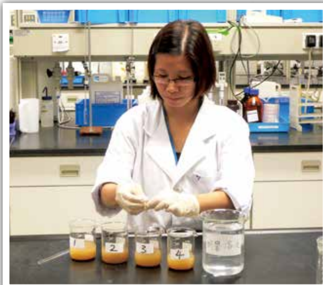
A laboratory technician is adding the alum solution into the beakers.
