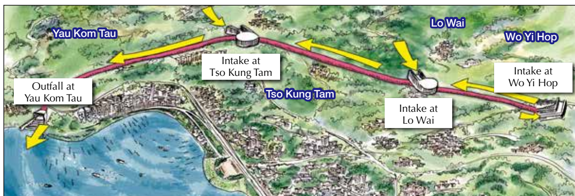
A sketch of the Tsuen Wan Drainage Tunnel
