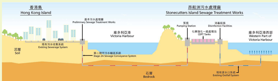
「淨化海港計劃第二期甲」 污水收集及處理過程之切面圖 Cross-section illustration of HATS Stage 2A sewage collection and treatment processes
