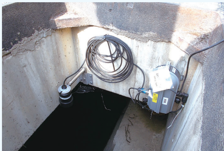
Data collection device (right) and ultrasonic sensor (left)
