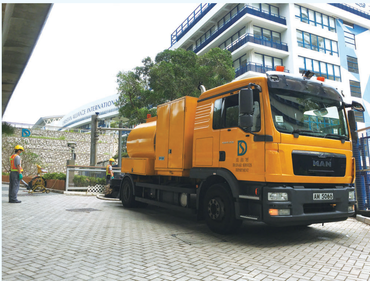
A high pressure water jetting unit uses rainwater harvested from a drainage tunnel for pipe cleansing in its daily operation
