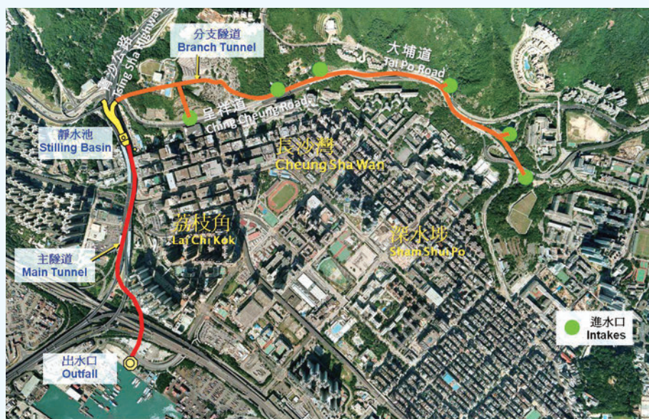
Lai Chi Kok Drainage Tunnel Layout Plan
