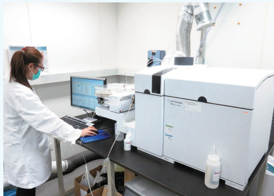
Inductively coupled plasma-optical emission spectrometer for detecting heavy metals in sewage and sludge samples
