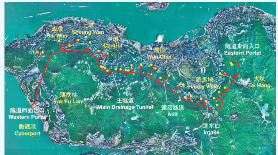
Hong Kong West Drainage Tunnel Layout Plan
