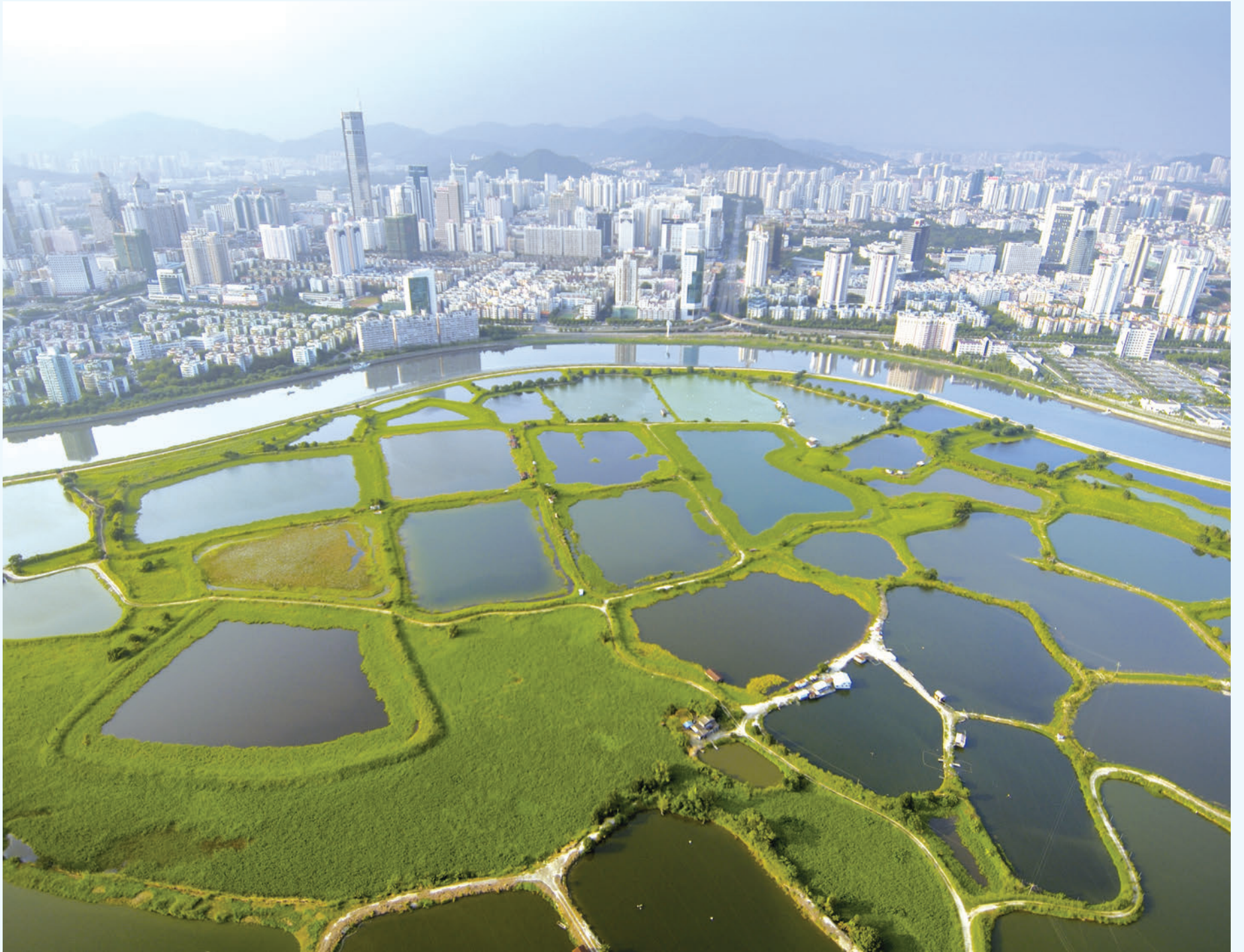
Section of Shenzhen River at Liu Pok downstream of the Lo Wu Control Point after river regulation to widen and straighten the river section
