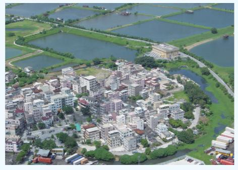
San Tin village flood protection scheme comprises a stormwater pumping station and flood storage pond, which can be seen at the top of this picture, and a ring road being part of the polder surrounding the low-lying villages.
