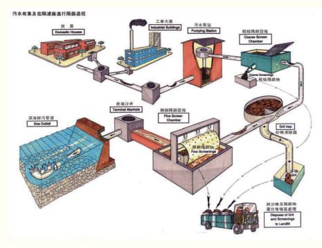
Typical operation flow within a preliminary treatment plant
