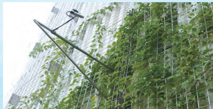
Infrared sensors on the exterior walls for temperature measurement
