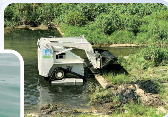
▲ 無線遙控清淤機械人 Wireless Remote-controlled Desilting Robot
