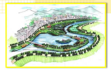
Use of flood retardation pond for flow attenuation
