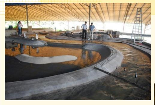
Simulates flow patterns inside the Flood Retardation Pond
