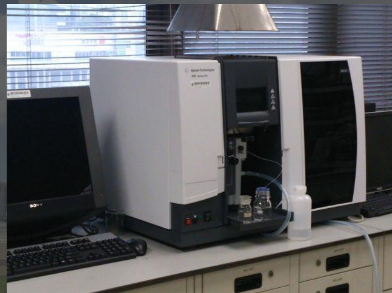
Atomic Absorption (AA) Spectrometer used for heavy metal analysis
