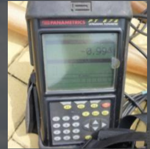
Runoff experiment setup (left) and ultrasonic flow meter (right)
