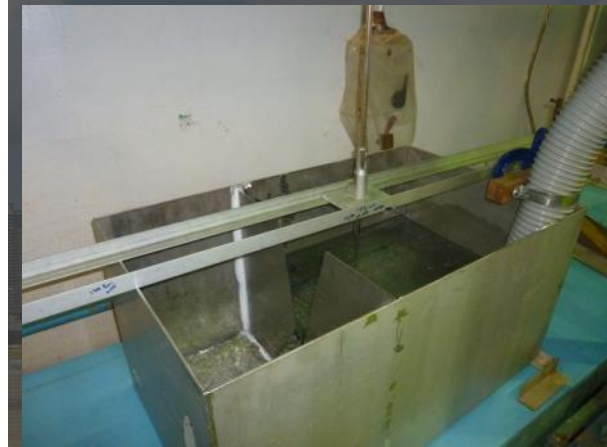
V-notch calibration setup in Hydraulics Laboratory
