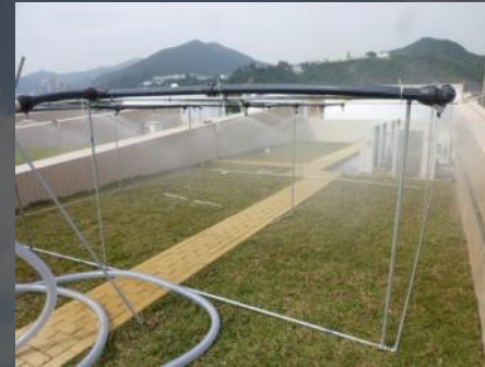
Runoff experiment setup (left) and ultrasonic flow meter (right)
