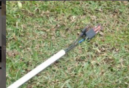
Soil temperature and moisture sensor (right) and data logger (left)
