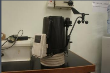
Weather station sensor suite
