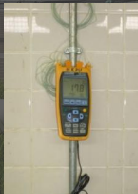
Thermocouple and data logger
