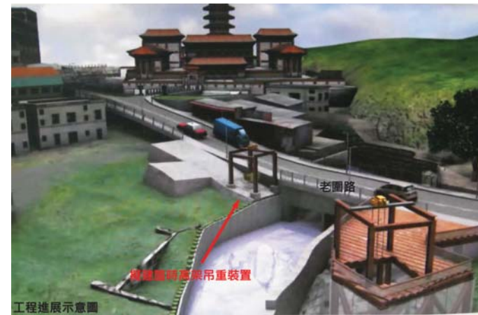
Illustration of the construction of man access shaft 興建維修人員通道工程示意圖
