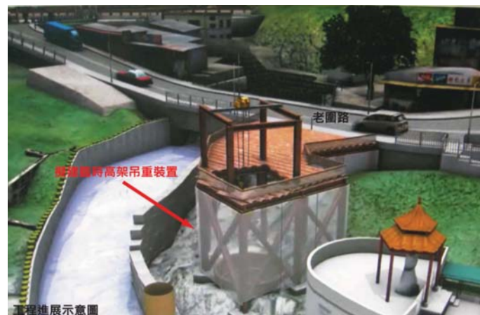
Illustration of the construction of vortex shaft 興建漩渦式引水渠工程示意圖
