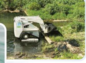
▲ 無線遙控清淤機械人 Wireless Remote-controlled Desilting Robot
