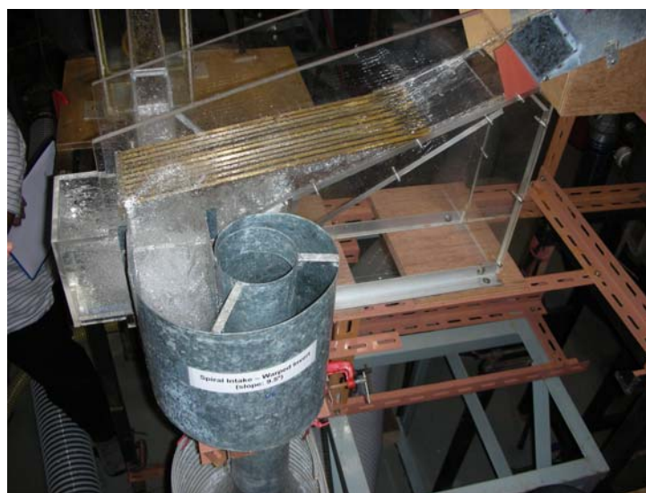
Figure 5 Physical Model Testing used to assess hydraulic performance of Intakes
