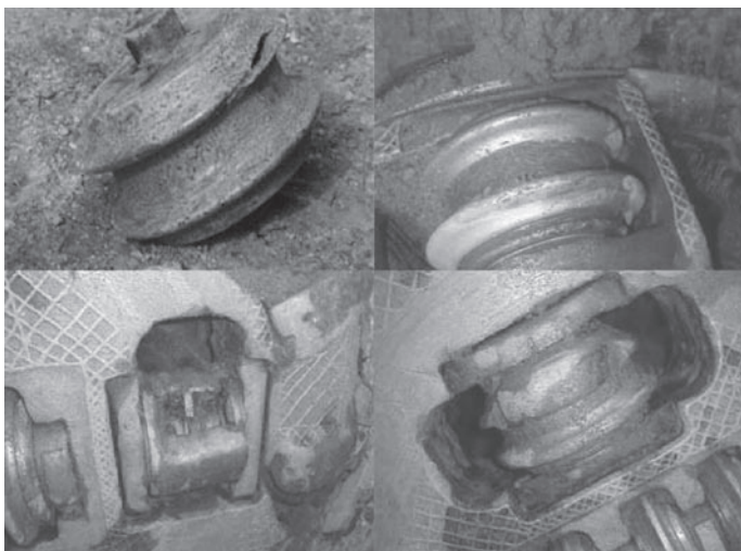
Figure 23 – Conditions of Damaged Disc Cutters
