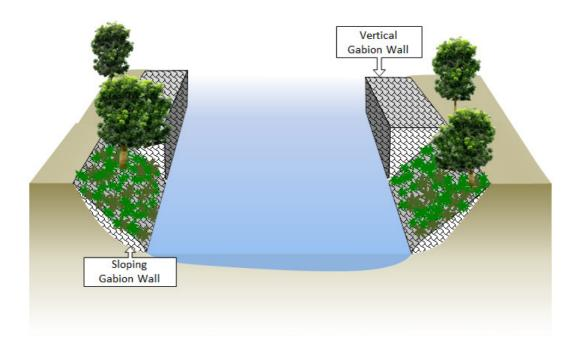
FIGURE 34 THE DIFFERENCE IN VEGETATION RE-COLONIZATION PERFORMANCE OF SLOPING GABION AND VERTICAL GABION
