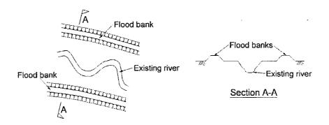
FIGURE 3 TYPICAL ARRANGEMENT FOR DISTANT FLOOD BANKS
