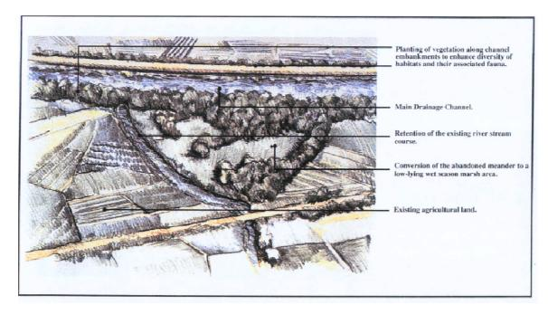
FIGURE 10 PRESERVATION AND ENHANCEMENT OF CUT-OFF MEANDERS (SOURCE: EXAMPLES OF ENVIRONMENTALLY FRIENDLY DRAINAGE CHANNEL ARISING FROM ENVIRONMENTAL IMPACT ASSESSMENTS BY EPD, DSD, AFCD & TDD)
