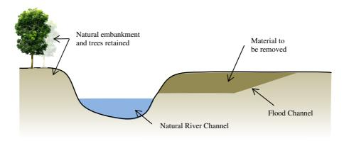
FIGURE 7 ALTERNATION OF WORKS
