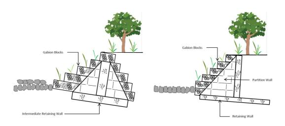
FIGURE 35 COMPOSITE STRUCTURE OF CONCRETE RETAINING WALL WITH GABION LINING
