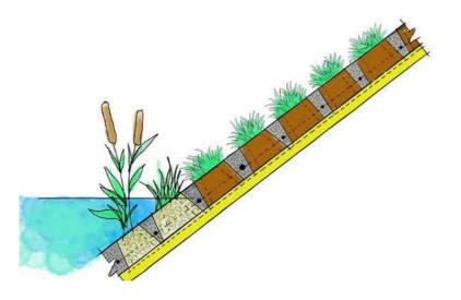
FIGURE 39 GRASSED CELLULAR CONCRETE PAVING AT EMBANKMENT
