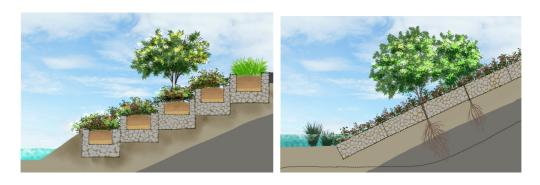
FIGURE 33 GABION BASKETS WITH PLANTING PITS (LEFT) AND VEGETATED GABION MATTRESS (RIGHT)
