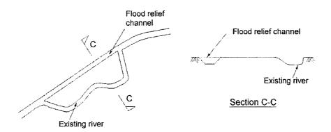
FIGURE 5 TYPICAL ARRANGEMENT FOR FLOOD RELIEF CHANNEL
