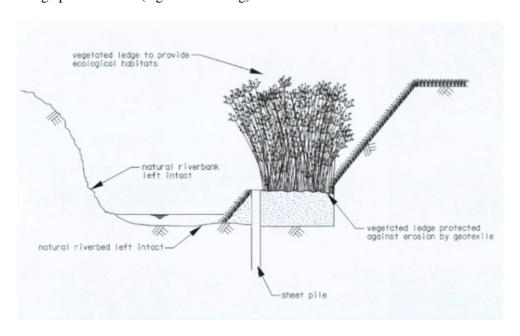
FIGURE 16 CREATION OF VEGETATED LEDGE BY SHEET PILES
