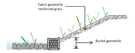
FIGURE 37 GEOTEXTILE REINFORCED GRASS EMBANKMENT
