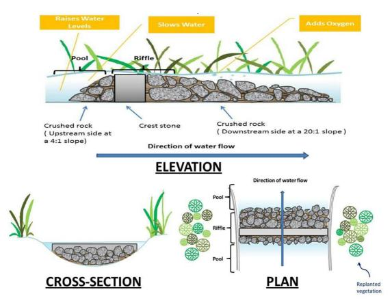
FIGURE 14 PLAN, ELEVATION AND CROSS-SECTION VIEWS OF A BOULDER WEIR AND ITS MAIN FUNCTIONS
