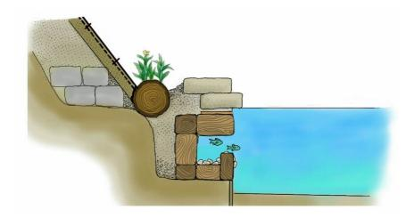
FIGURE 28 AN UNDERCUT BANK TO PROVIDE FISH SHELTER
