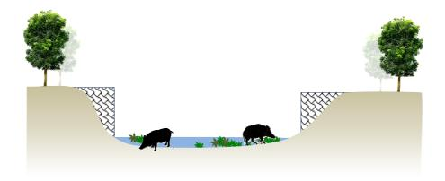
FIGURE 8 ANIMALS COULD BE TRAPPED IN CHANNEL WITH VERTICAL EMBANKMENT WITHOUT PROVISION OF ANIMAL CORRIDOR
