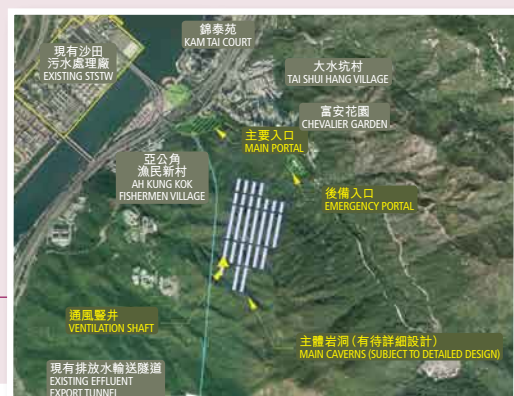
搬遷沙田污水處理廠往岩洞的初步佈局 Preliminary layout of Relocation of Sha Tin STW to Caverns
