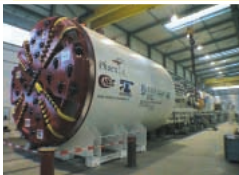
啟德雨水轉運計劃鑽挖機的鑽頭 Drilling head of boring machine for Kai Tak Transfer Tunnel
