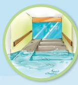
Elevate entrance / floor levels, or install door sills / steps, especially at pedestrian and vehicular entrances to basements.
