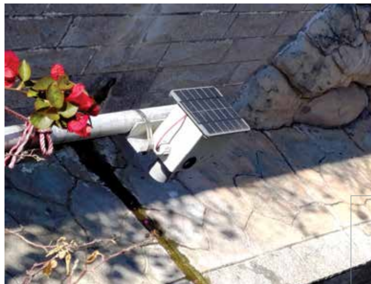
部分新型傳感器可由太陽能供電 Some new sensors can be powered by solar energy
